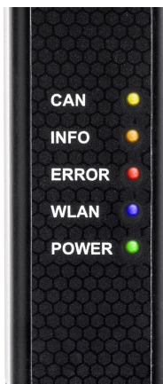
Figure 3: LEDs on the Kvaser BlackBird Pro v2.
