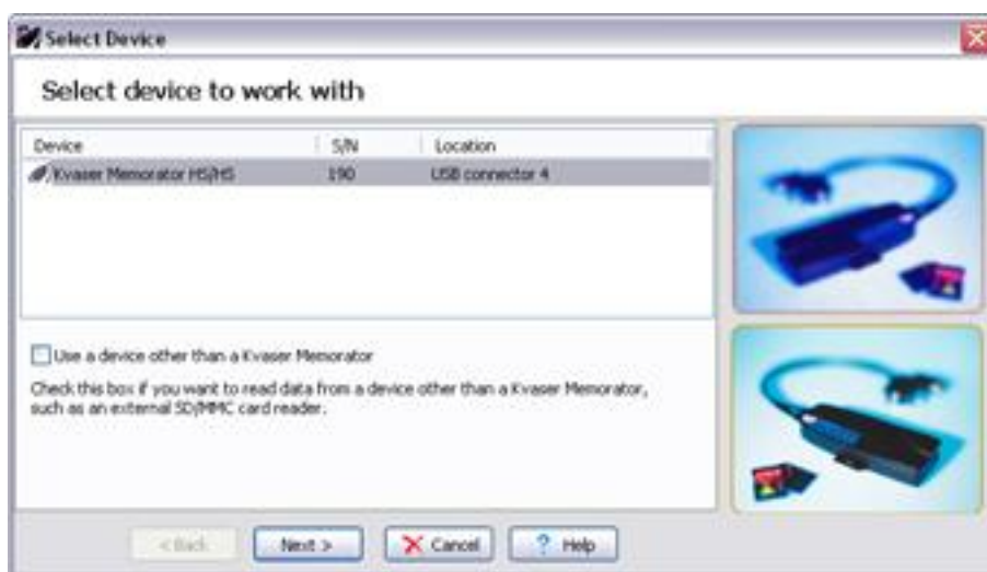
Figure 4: How to connect a Kvaser Memorator to the setup tool.
