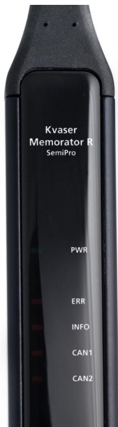
Figure 3. LEDs on the Kvaser Memorator R SemiPro.
